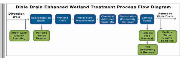
Water up to the peak design water flow rate (200 cfs) will be diverted from Dixie Drain near the southern corner of the property into the sedimentation basin to begin the treatment train process. A diversion structure will be installed in the drain to convey water into the treatment system. Operable gates are planned to control the amount of water that is diverted through the treatment system.
